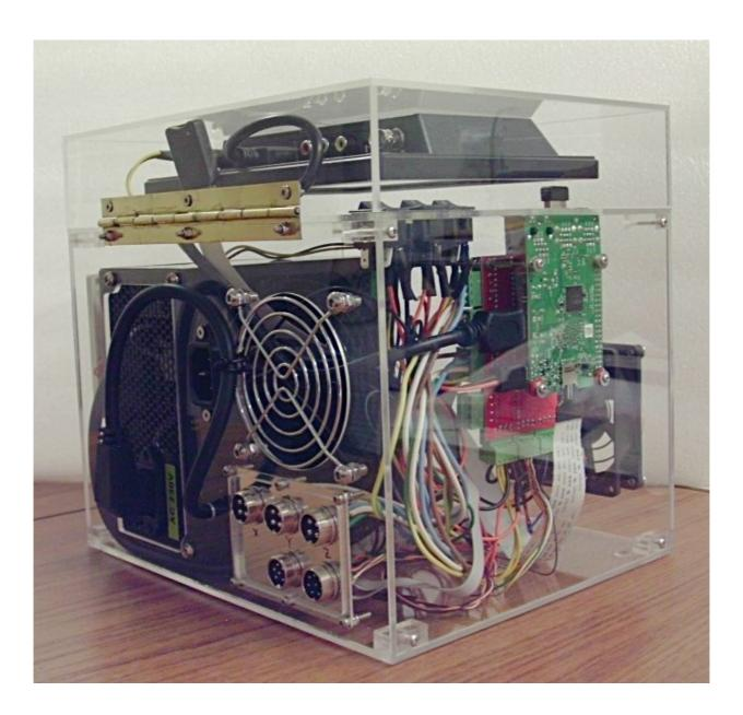
The program that does all the hard work on the Raspberry Pi is called "bCNC". It can create G code from scratch or from DXF files. It can visualise the G code in 2D or 3D and, most importantly, it feeds the G code to the Protoneer GRBL controller and produces real-time feedback on screen. It can also handle tool changes, probing in multiple directions and auto-leveling which is very useful when routing printed circuit boards.
